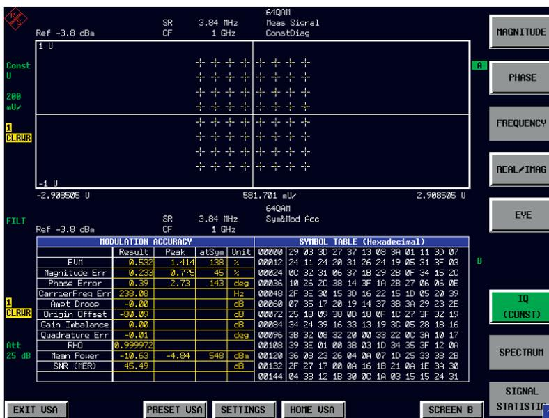
Convenient analysis with the vector signal analysis option (R&S®FSQ-K70): The upper part shows the constellation diagram of a signal with 64QAM modulation. The table below lists the most important parameters for characterizing a signal with digital modulation, including the demodulated bits.
