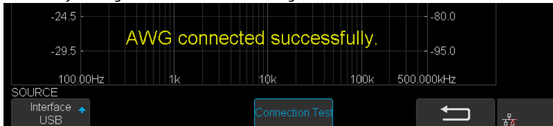
Figure 139 Bode Plot Interface Connection
