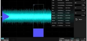
The Waveform Histogram feature provides a statistics view of the waveform in horizontal and vertical directions
