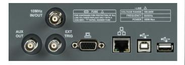
USB Host, USB Device (USBTMC), LAN (VXI-11, telnet, socket, web), Pass/ Fail, Trigger Out, 10 MHz In/Out and VGA output
