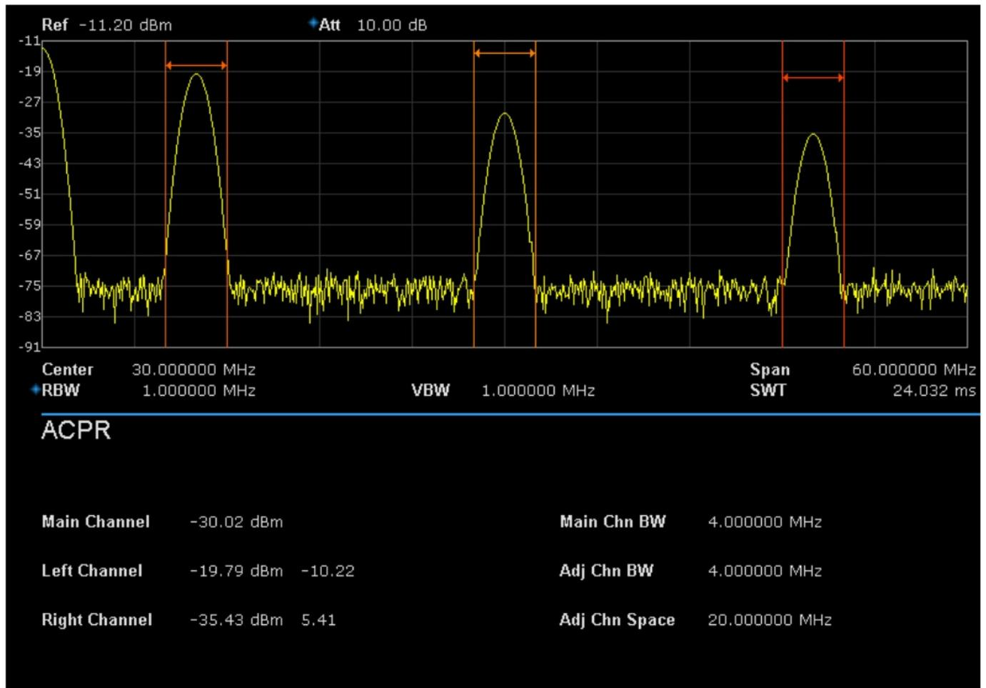
**Adjacent Channel Power Measurement:** Main CH Power, Left channel power and Right channel power.
