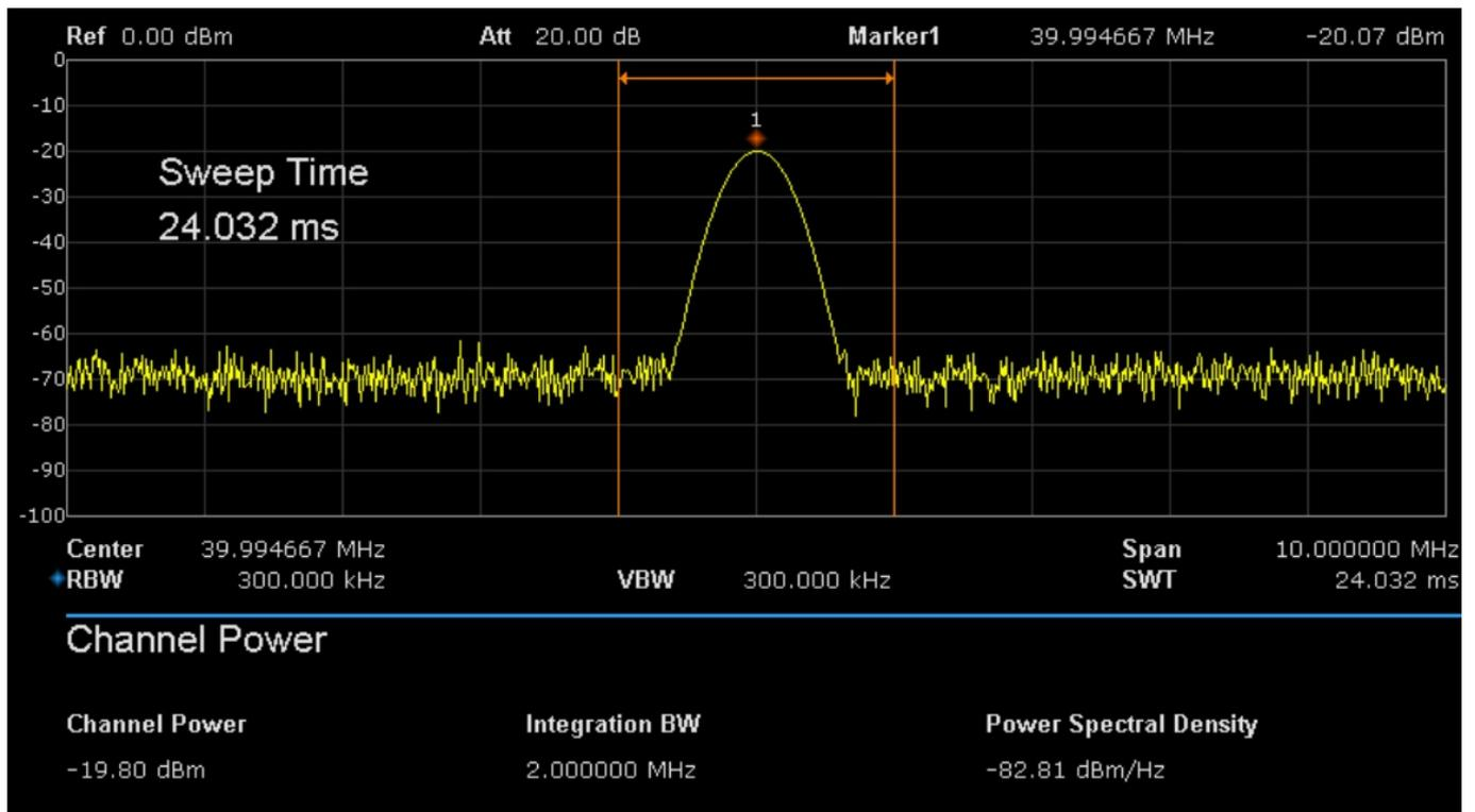
**Measurement Results:** Channel power and power spectral density.
