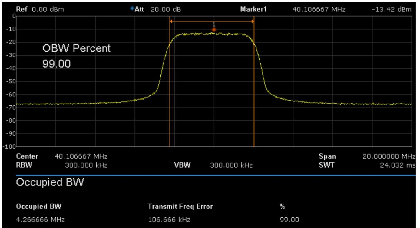
**OBW measurement:** Occupied bandwidth and transmit frequency error.
