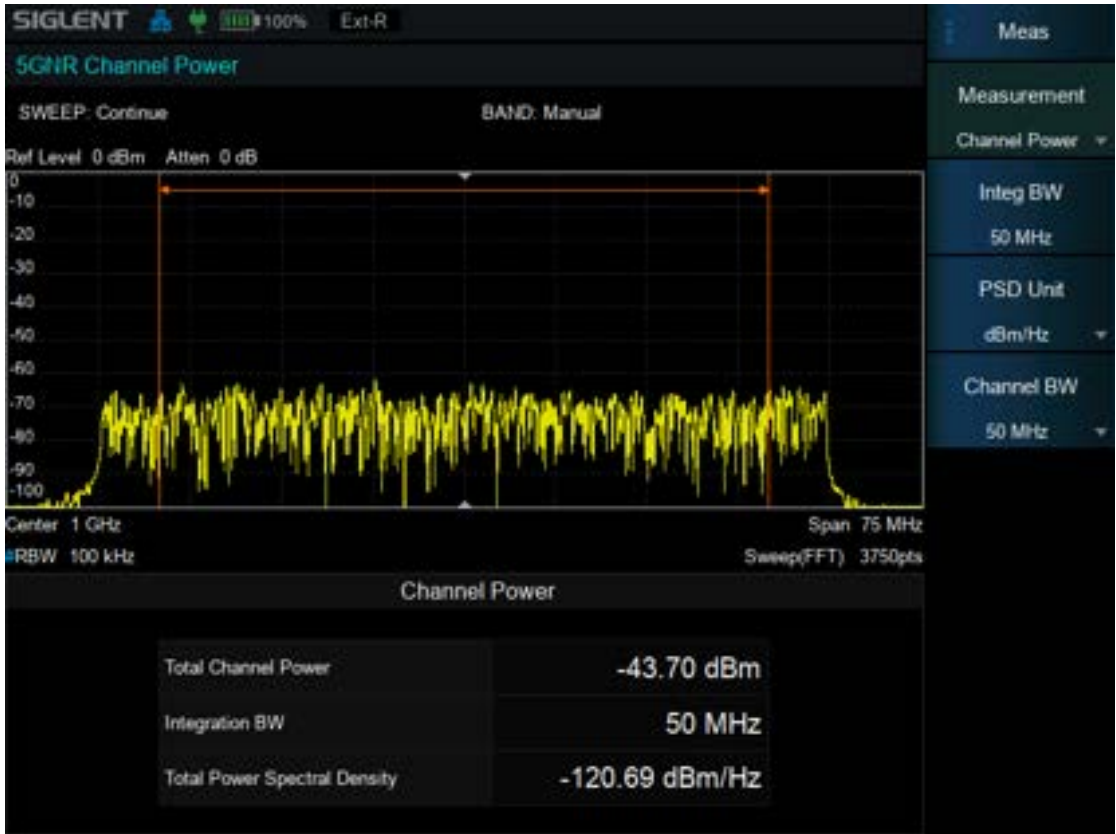
Figure 8–5 Channel power view
