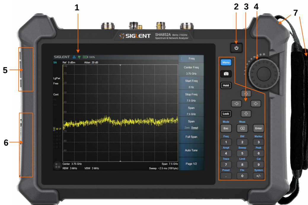
Figure 1–4 the Front Panel
