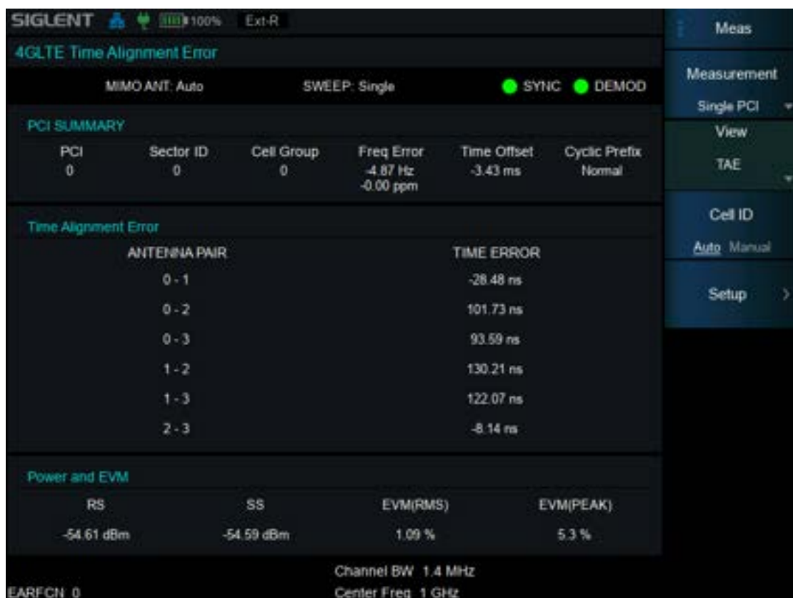
Figure 9–2 Single PCI TAE view
