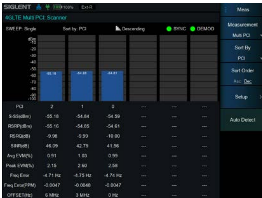
Figure 9–3 Multi PCI View
