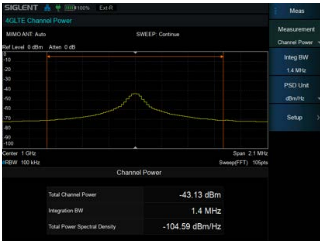
Figure 9–4 Channel Power View
