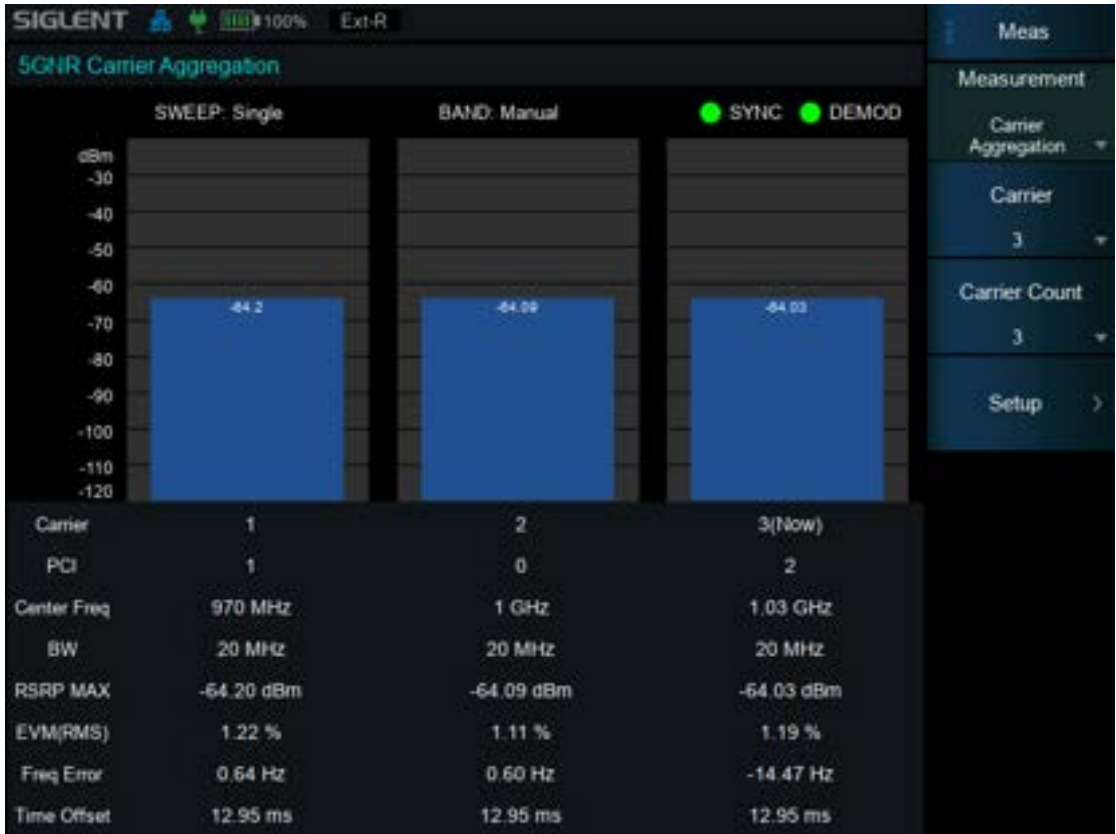
Figure 8–7 Carrier Aggregation View
