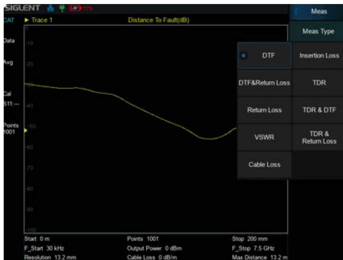
Figure 2-3 CAT measurement selection
