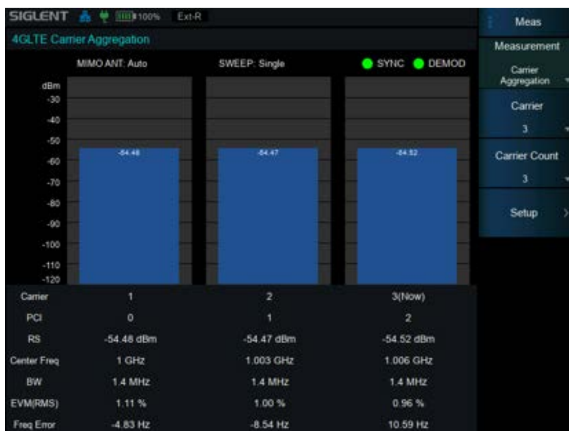
Figure 9–6 Carrier Aggregation View
