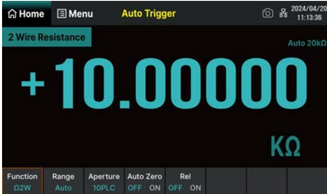
Figure 7-13 2-Wire resistance measurement interface
