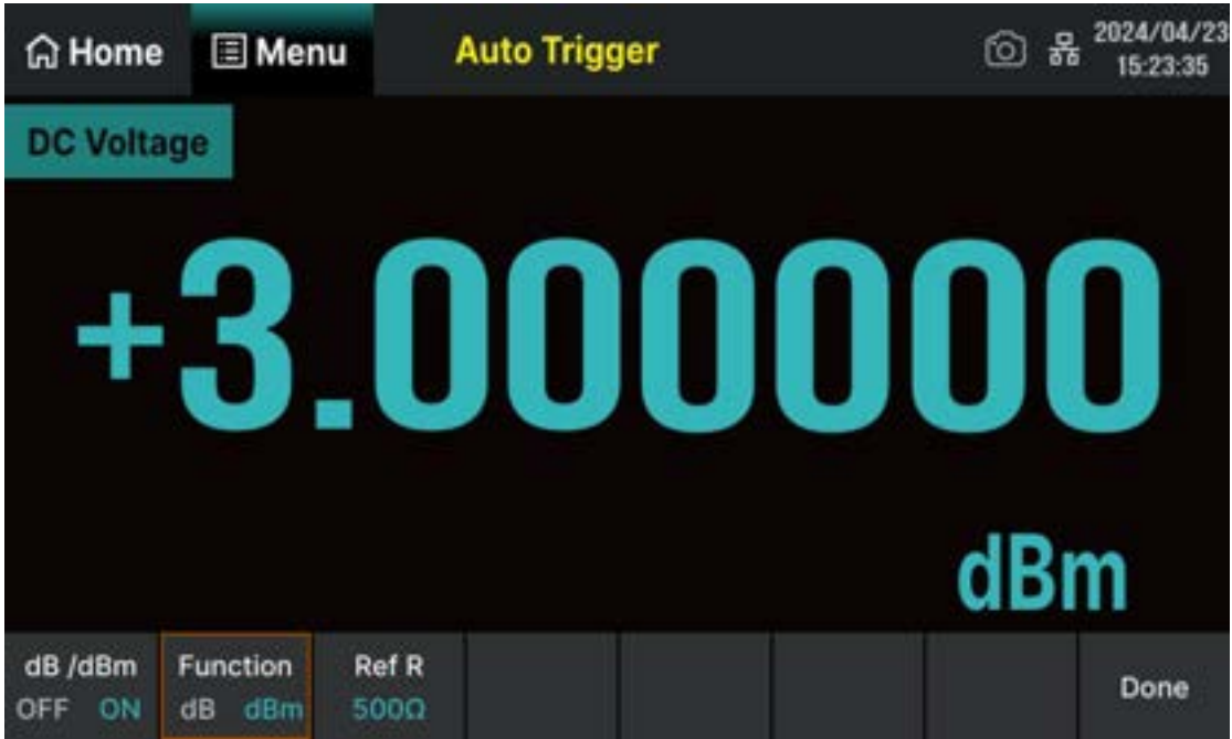
Figure 7-54 dBm function menu interface
