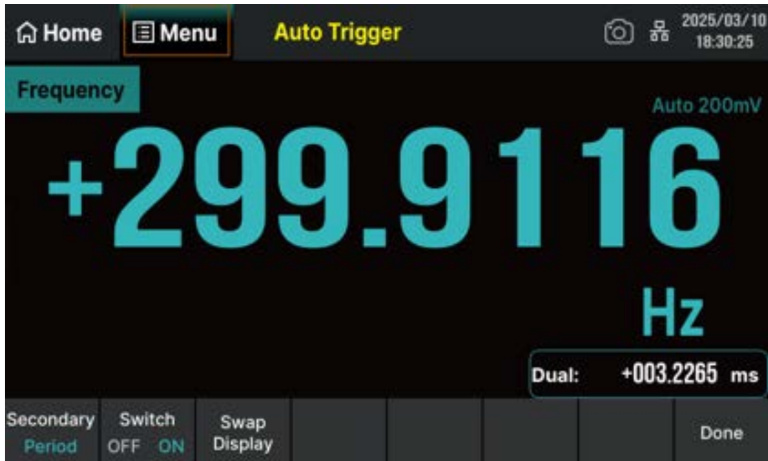
Figure 7-30 Dual-display interface (main display – Freq, secondary display – Period)
