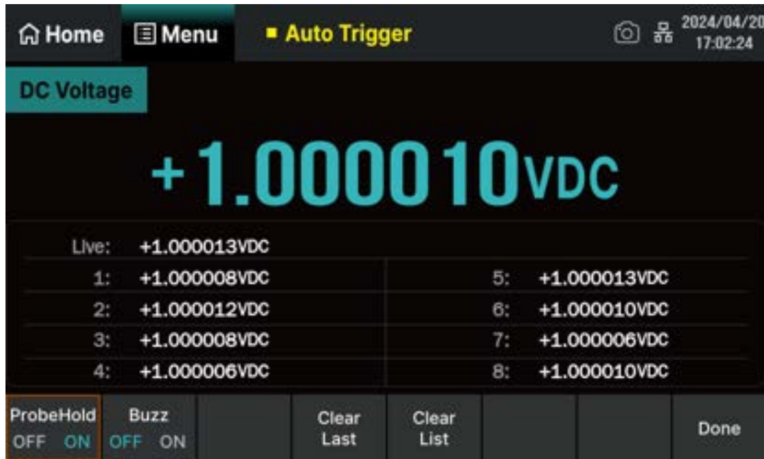
Figure 7-61 Probe Hold function interface
