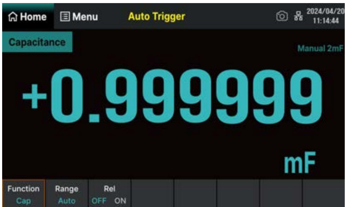
Figure 7-15 Capacitance measurement interface
