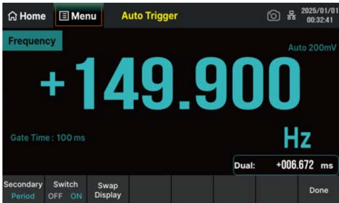
Figure 7-28 Dual-display interface (main display – Freq, secondary display – Period)
