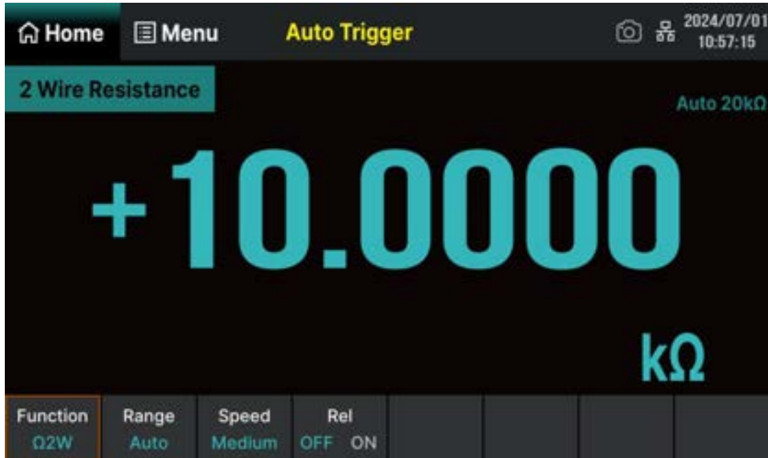
Figure 7-11 2-Wire resistance measurement interface
