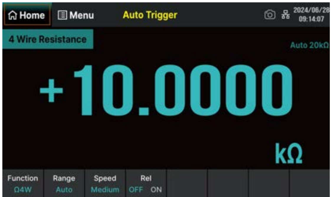
Figure 7-12 4-Wire resistance measurement interface
