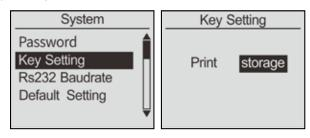
Set the default function of the "LOG" key from the home screen. The function can be set to print or store the current displayed value. Press "ZERO" or "MODE" to select the proper setting. Press "LOG" to cancel; touch "MENU" to confirm and exit. The default value is set to Storage
