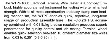
The WTPT provides long operation life and power flexibility with the ability to work from the internal rechargeable battery or included AC adapter. The analog bar graph on the backlit, LCD aids users by providing the resultant force's current position compared to the full-scale range.
