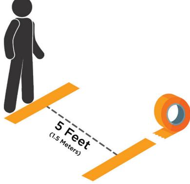
**2.** Place two pieces of tape 5 feet (1.5 m) apart. Position is critical to system performance.
