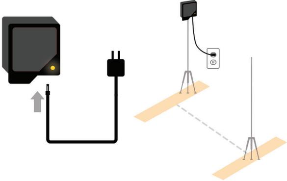
**4.** Heat source automatically turns on once plugged in. Ready when light stops blinking.
