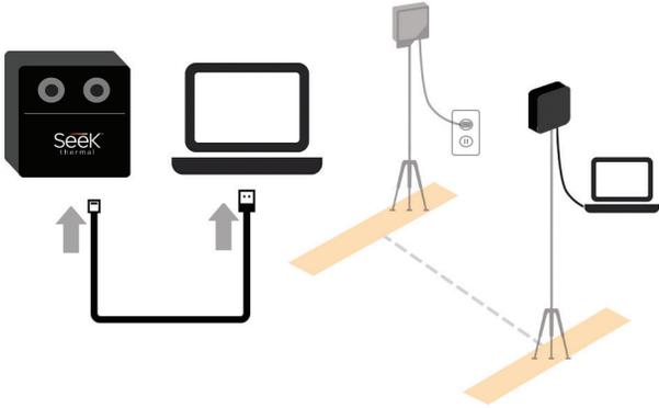
**5.** Attach camera to tripod and connect cable to PC or tablet. Software must be already installed.
