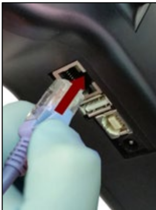
Figure 7. Connecting Ethernet Cable
