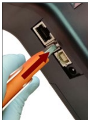
Figure 8. Connecting USB - A Host
