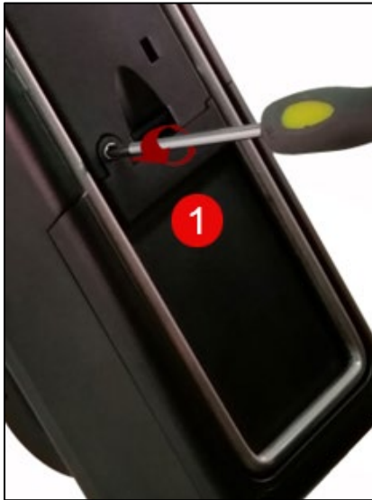
Figure 10. Install Battery Pack Step 1
