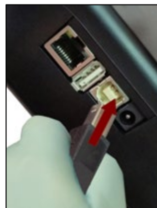
Figure 9. Connecting USB B Client
