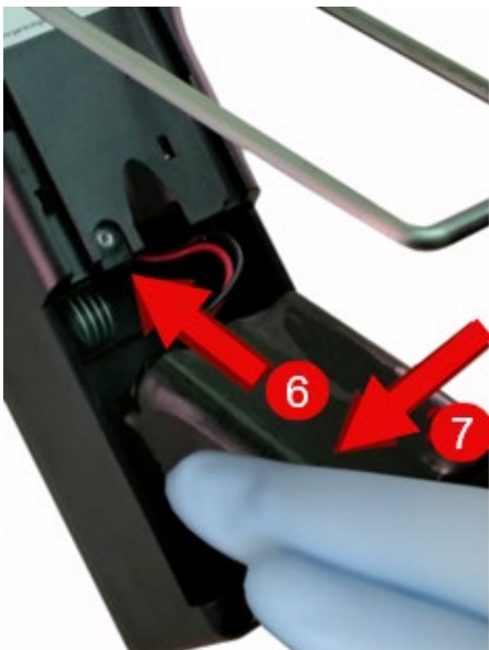
Figure 14. Install Battery Pack Step 5
