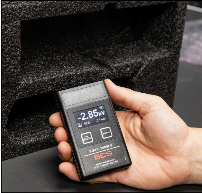
Figure 7. Using the Static Sensor to measure foam
