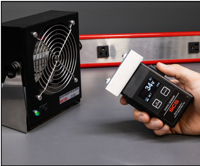
Figure 14. Measuring the offset voltage (balance) of an ionizer with the Air Ionizer Test Kit
