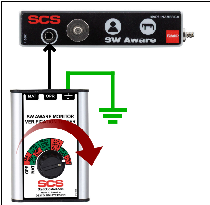
Figure 4. Connecting the 770153 Verification Tester to the SW Aware Monitor's operator jack
