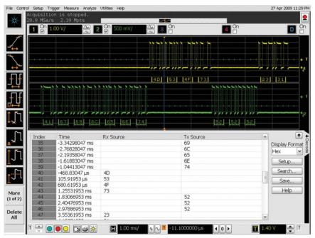
RS-232 protocol decode with precise time-correlation between waveforms and listing
