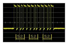
RS-232 decode embedded in waveform area
