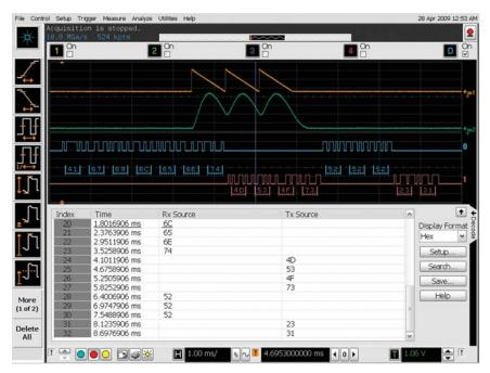
Use digital channels on MSO models to preserve analog channels for simultaneously viewing other signals..
