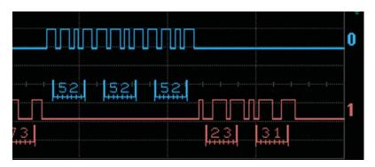
See RS-232 decode next to digital waveforms.
