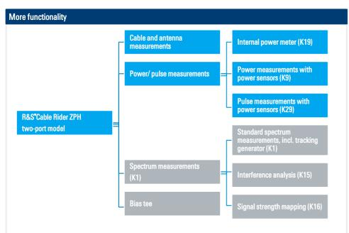
Functions in blue boxes are available for the R&S®Cable Rider ZPH one-port and two-port models. Functions in green boxes are available ONLY for the R&S®Cable Rider ZPH two-port model.
