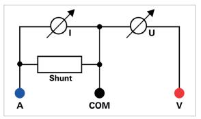
Fig. 4.4: Internal wiring of A, V and COM jacks.
