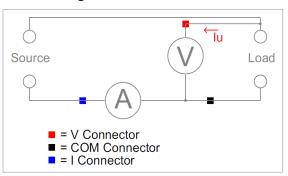
Fig. 4.5: Voltage-based measurement.
