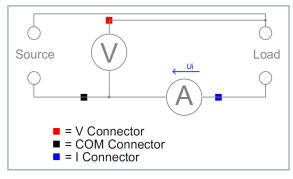
Fig. 4.7: Current-based measurement.
