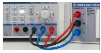
Fig. 4.8: Current-based measurement, wiring example.
