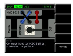
Fig. 6.14: HZC815 connection example EN 50564
