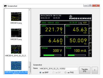
Fig. 8.3: Screenshot module of the HMExplorer Software
