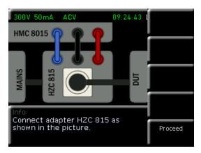
Fig. 6.17: HZC815 connection IEC 61000-3-2
