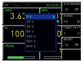
Fig. 5.8: Manual measurement range selection via ACQ menu
