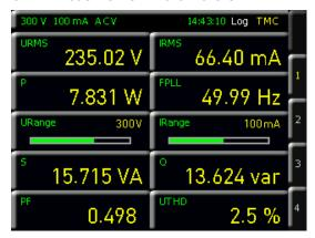
Fig. 6.1: R&S®HMC8015 readout display.
