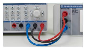
Fig. 4.6: Voltage-based measurement, wiring example.
