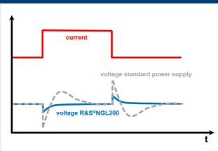
During challenging load conditions, most power supplies react with slow recovery times and overshoots. Specially developed circuits in the R&S®NGL200 series achieve a load recovery time of < 30  $\mu$ s with minimal overshoot, making them perfect for supplying sensitive components
