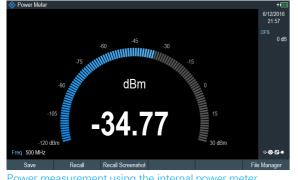
Power measurement using the internal power meter
