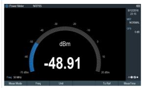
Power measurement with the R&S®NRP8S power sensor
