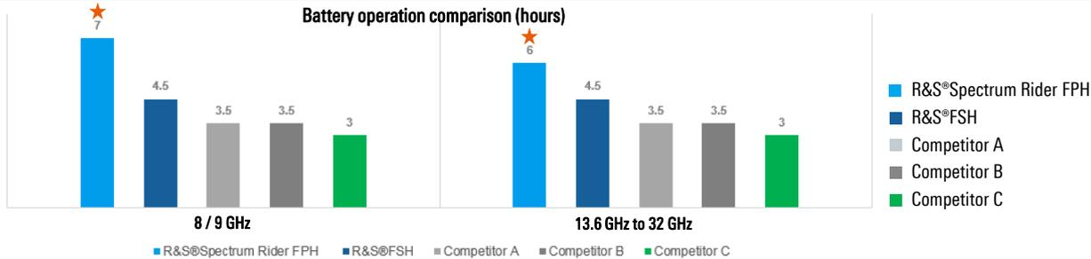
The analyzer has an innovative fanless concept – part of a rugged design that protects it from dust and water. Designed with power optimization in mind, the R&S®Spectrum Rider consumes less power than competitor products and can be operated for a full working day without recharging.
