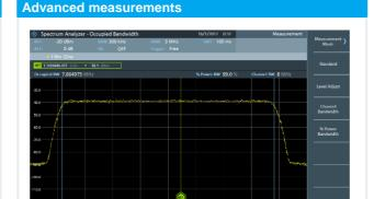
The R&S°FPC-K55 adds measurement functions for channel power, occupied bandwidth, spectrogram display, harmonic distortion, TDMA power and third order intercept.
