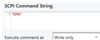
Figure 4-159: Example for the Identification command of a generic amplifier (here: from manufacturer "Bonn", which is shown as an editable Required Substring in Answer)
