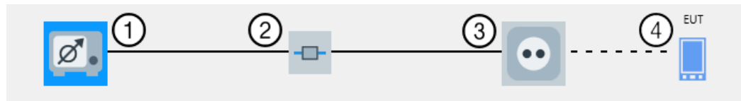
Figure 4-131: EMI conducted hardware setup diagram LISN
