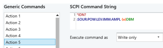
Figure 4-160: Color-coded parts of a SCPI command
