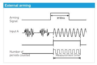
External arming prevents undesired signals from triggering of a measurement.
