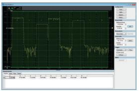
Measurement of eight timeslots in one shot with the R&S $^{\circ}$ NRPV.
