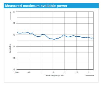
The high output power of typ. > +17 dBm enables measurements on DUTs such as mixers that require a high level for the local oscillator.
