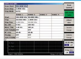
In receiver mode, the R&S\*ESL is tuned in fixed frequency steps in accordance with the settings in the SCAN table. The SCAN table can be programmed for a maximum of ten frequency subranges with independently selectable parameters.
