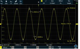
QuickMeas: automatic measurement and graphical display at the push of a button.
