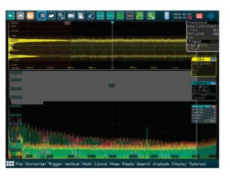
R&S®RTE oscilloscopes come with built-in spectrum analysis for up to four signals in parallel. Results can be correlated in the time and frequency domain. Analysis functions such as spectrogram (with R&S®RTE-K18 option), mask test and peak list are available.
