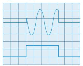
Output signal controlled by a gate signal).
