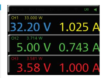
The different operating conditions are marked by colors: constant voltage operation is indicated in green, constant current operation in red, inactive channels are shown in yellow, blue indicates that the channel is in setting mode.
