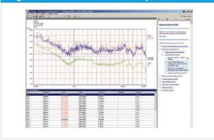
Preview measurement (Pk and Avg) with determination of the local maxima (here, 25 subranges) for subsequent final measurement (QP and C-Avg).
