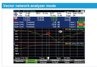
For cable loss and antenna testing and characterization as well as distance to fault measurements.
