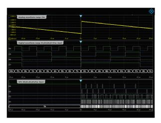
With the R&S®RTE-B1 option, every R&S®RTE can be turned into a mixed signal oscilloscope with 16 digital channels. This example shows the ramp signal of a 4-bit ADC with analog and digital channels correlated to an SPI bus that controls the ADC.
