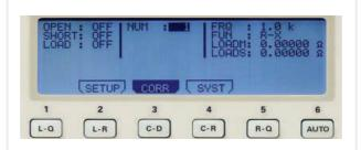
Activation and deactivation of OPEN, SHORT and LOAD correction.
