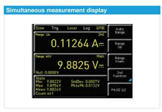
Simultaneous display of three measurements, including DCI and ACI at the same time.
