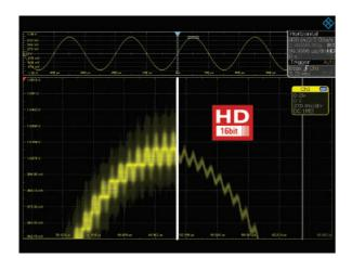
The high definition mode (HD mode) increases the vertical resolution of the R&S\*RTE to up to 16 bit. This results in sharper waveforms, showing signal details that would otherwise be masked by noise.
