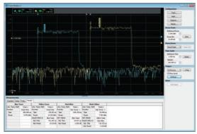
Pulse delay measurement on different traces.
