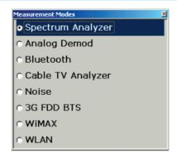
The R&S®FSL offers many different firmware options. The user can switch between different applications.
