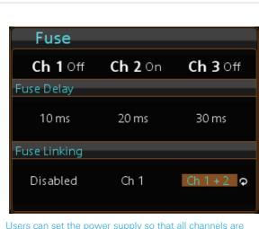
Users can set the power supply so that all channels are switched off if one channel hits the limit. Or it can be set to leave one channel working.
