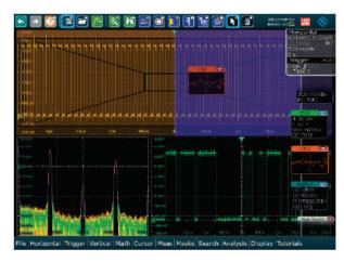
You can drag & drop waveforms and result windows on the screen. The SmartGrid function helps you flexibly arrange multiple diagrams on the screen.
