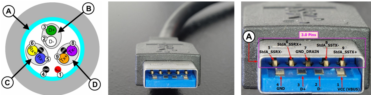
Figure 13-44: USB 3.1 cable cross-section and Standard-A plug - backward compatible with USB 2.0
