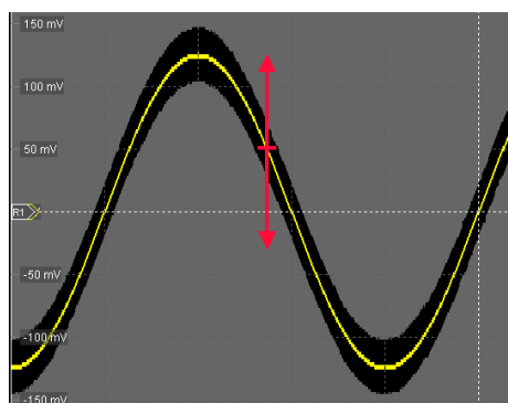
Figure 10-3: Waveform mask with vertical width = 0.5 div
