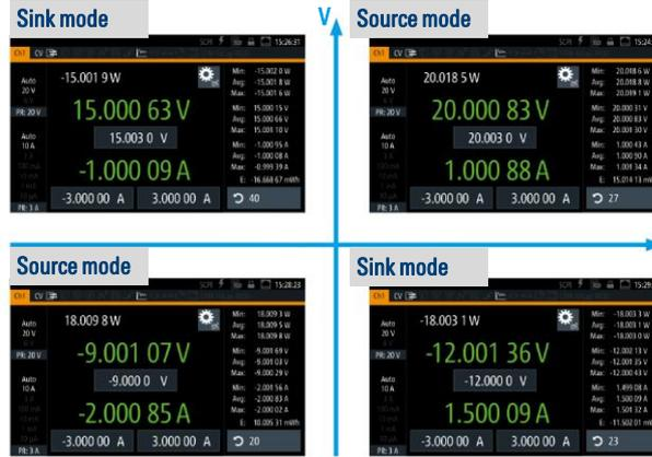
With its four-quadrant architecture, the R&S®NGU401 can supply positive and negative voltages and currents and can act as a source or sink in both polarities.
