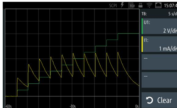
In this example, the charging current of a capacitor is displayed while the voltage is increased stepwise.
