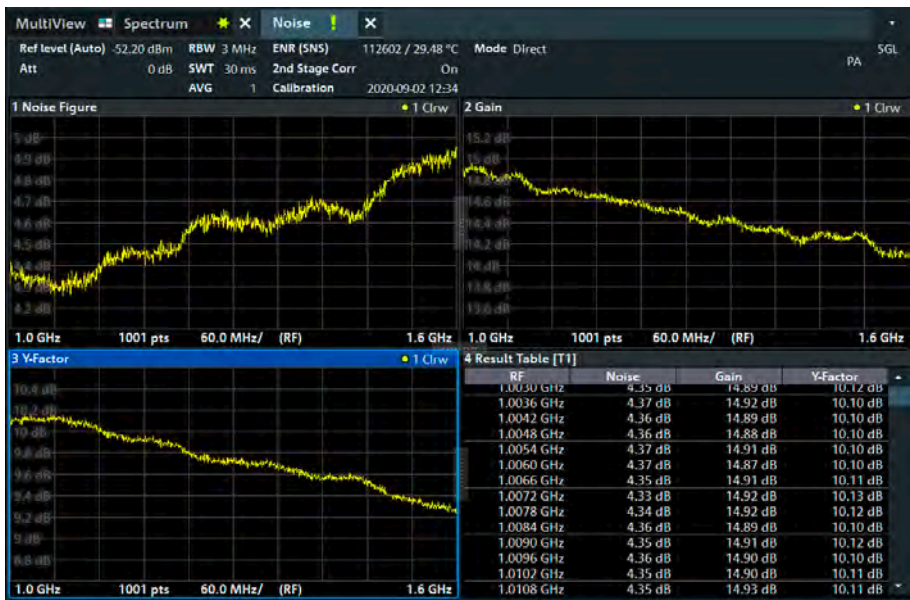
Simultaneous view of graphs for noise figure, gain and Y-factor versus frequency and a table of the results in numerical format
