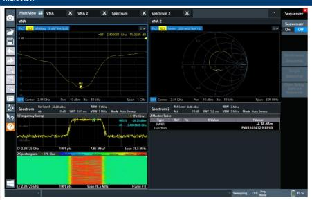
MultiView provides a convenient overview of all active R&S®ZNL modes. Here you see the combination of spectrum analyzer and network analyzer. In this view, all modes can be updated sequentially.
