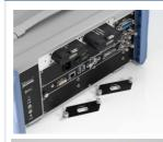
With batteries, the R&S°ZNL can be used outside the labs. Batteries are hot-swappable.
