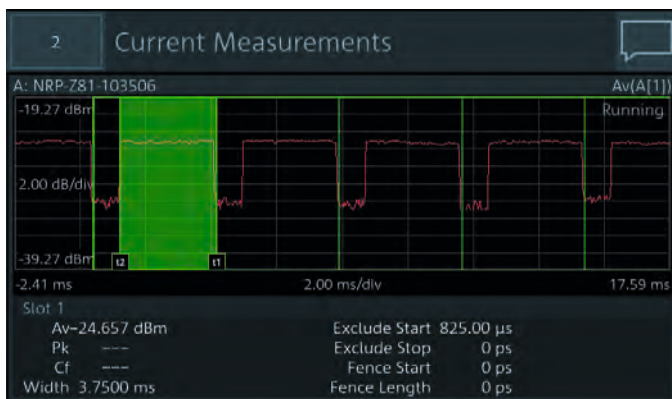
Timeslot measurement of a Bluetooth® signal with exclude start time
