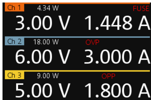
Figure 5-13: Indicator of OVP/OPP when tripped
