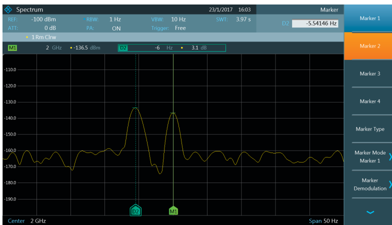
R&S®FPC-B22: high sensitivity with 1 Hz resolution bandwidth.
