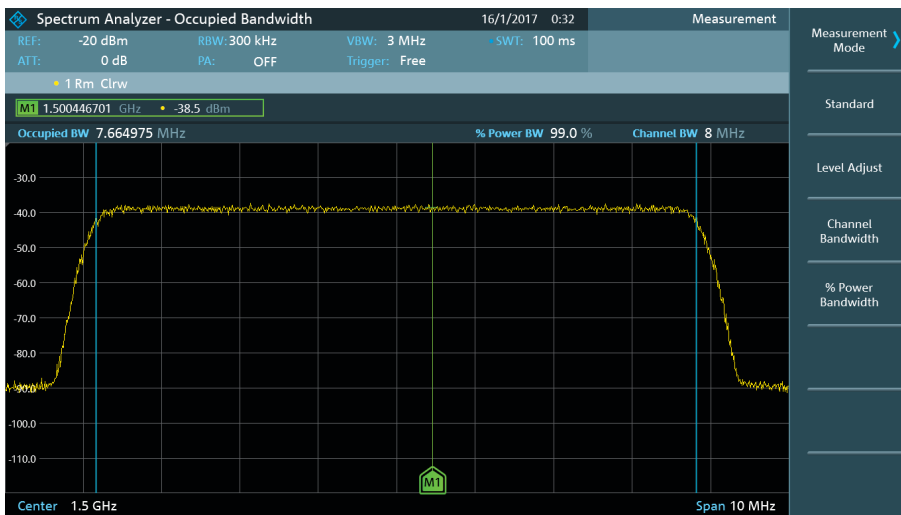
R&S®FPC-K55: occupied bandwidth.
