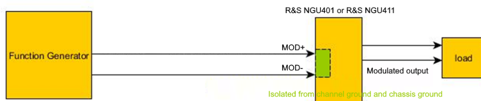
Figure 6-23: Setup of amplifying for modulating input source
