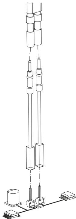
To use the standard square headers also for current measurements, you can use adapter cables to 2.54 mm delivered within the option R&S RT-ZA36, see [Table 2-9](#). The PCB adapters are designed for current measurements of only up to 3 A. These adapter cables are recommended for external shunt measurements.
