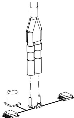
To reduce burden voltage, use the external shunt for the measurements of higher current drains. The figure shows the solder-in connection of external shunt.
