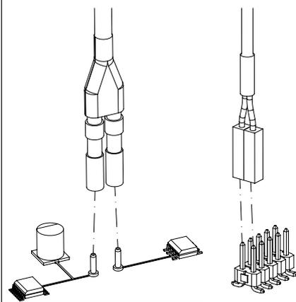
The headers soldered to the DUT provide firm contact with the measurement point during the whole measurements. The signal lead is plugged onto soldered-in headers on the DUT.
