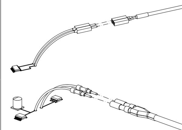
The PCB cables provide a flexible connection to the DUT. They are soldered onto the DUT and connected with the signal lead.
