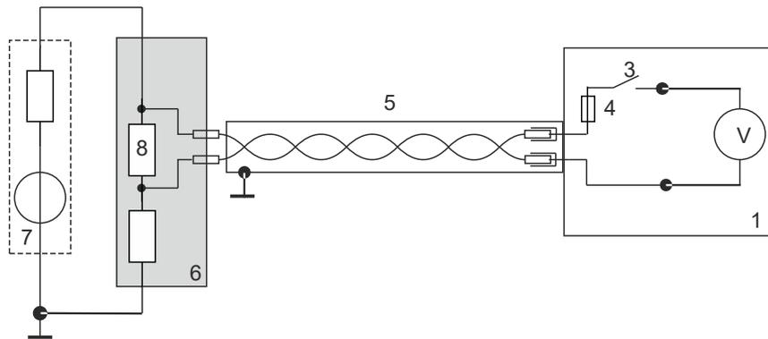
**Figure 4-6: Scheme of the shunt-ammeter with external shunt**
