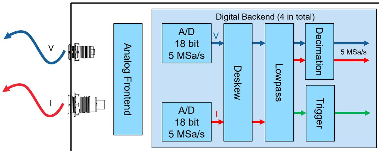
Figure 4-3: Signal flow with an oscilloscope
