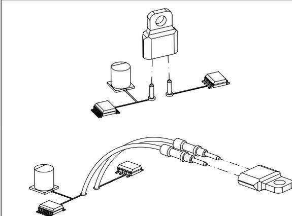
If the current measurement points are temporarily not connected to the probe box, close the circuit at the DUT via delivered shorting links. The figure shows shorting links connected to soldered-in headers (top) and PCB cables (bottom).
