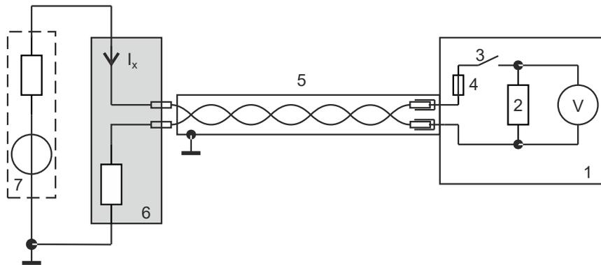
**Figure 4-5: Scheme of the shunt-amperemeter with internal shunt**
