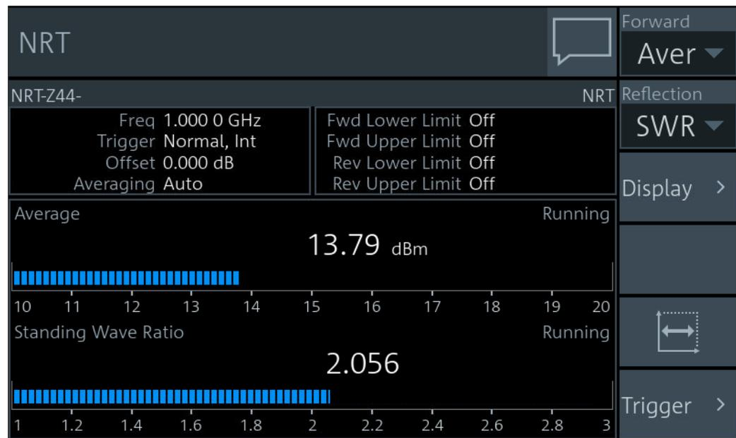
Displays two scalar values. One for the selected **Forward** measurement and one for the **Reflection** measurement.
