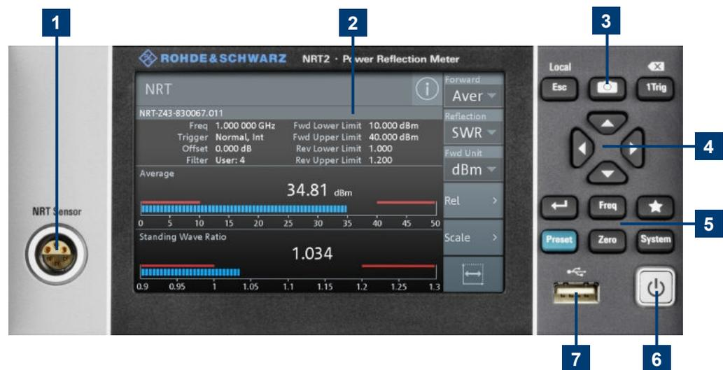
**Figure 3-2: Front panel of the R&S NRT2**
