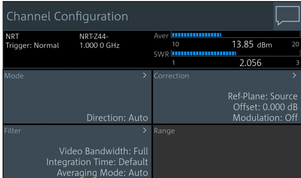
An R&S NRT-Zxx directional power sensor has two measurement channels, one channel for forward power and one channel for reflected power.
