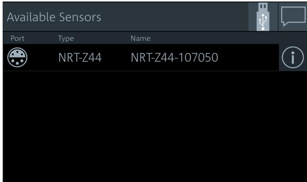
The R&S NRT2 displays the recognized sensors.
