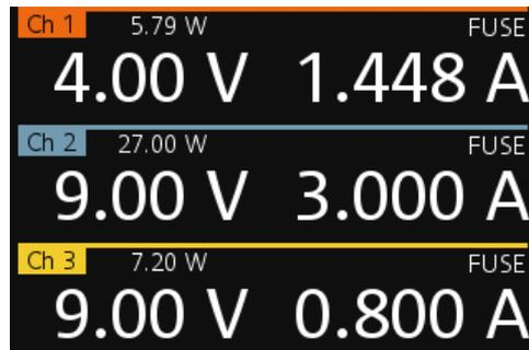
Figure 7-4: Fuse indicator on respective channel
