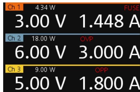
Figure 7-7: Indicator of OVP/OPP when tripped
