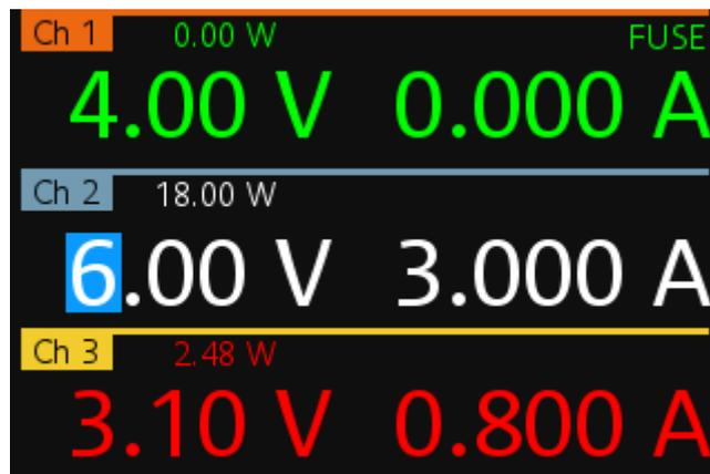
Figure 5-10: Color coding of difference operating conditions
