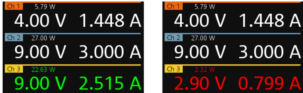
Figure 7-3: Output of Ch 3 in CV and CC mode
