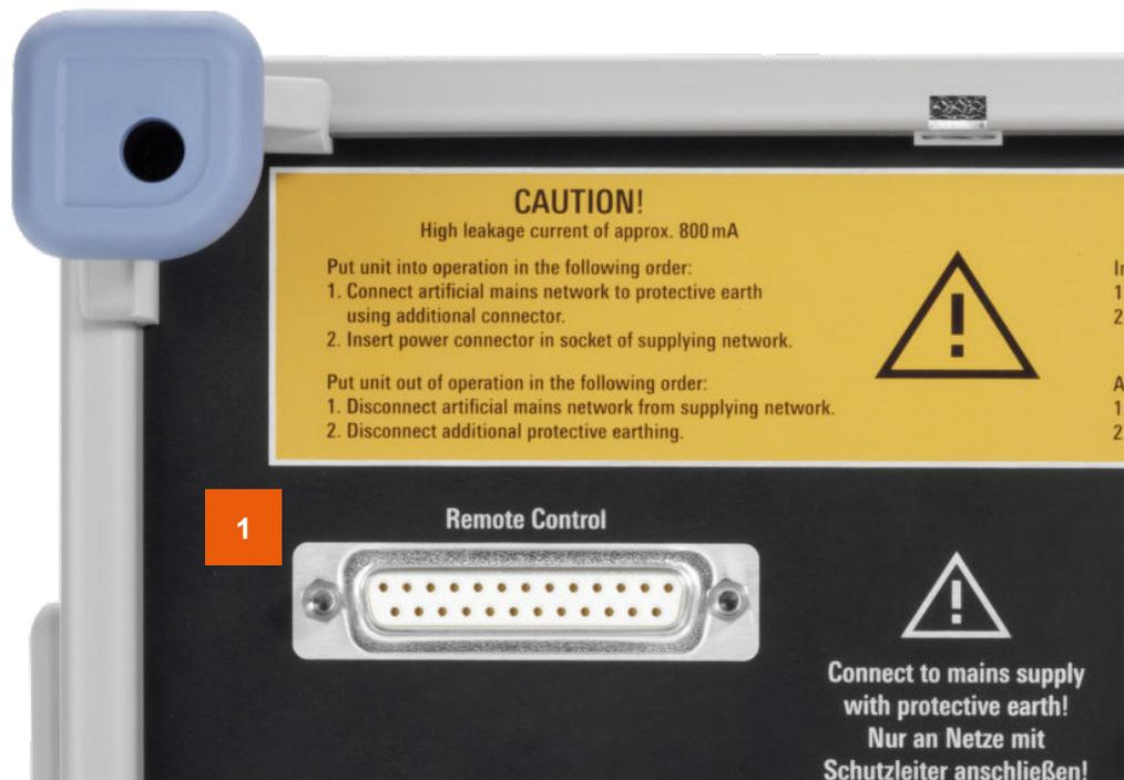
When a LOW signal is detected at input L1, N or 150 kHz HP, the corresponding function is activated and manual operation is blocked at the same time. The functions that have been switched on are indicated by the associated LEDs. When remote control is active, the REMOTE LED is lit.
