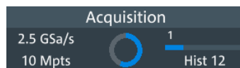
Figure 4-11: Progress of incomplete long acquisition in average mode, Run Single = 5, first acquisition is finished
