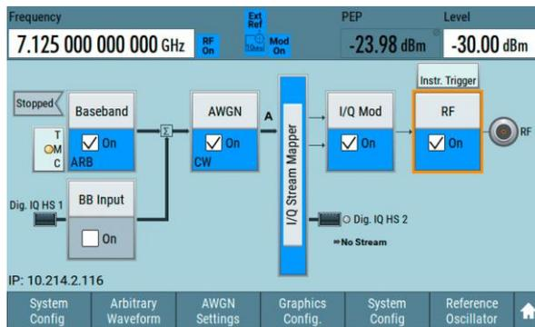
Instantly see the signal flow in the R&S®SMCV100B as well as the status of instrument inputs and outputs. An integrated graphic function displays the generated signal in real time.
