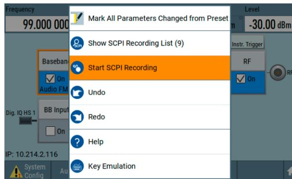
The integrated SCPI macro recorder has a built-in code generator that allows users to automatically record all manual settings and create a directly executable MATLAB® script.
