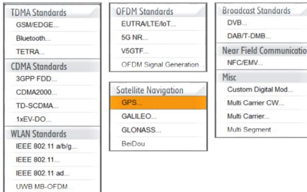
Modulated signals for different standards can be generated with the R&S®WinIQSIM2™ simulation software. The software supports wireless standards such as 5G and LTE and the generation of noncellular signals such as Wi-Fi (IEEE 802.11x) and many others.
