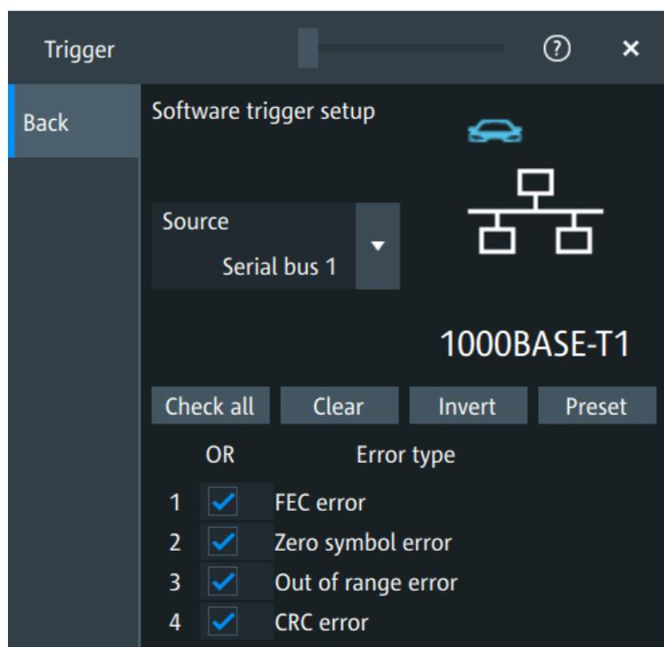
The following error types are available: "FEC error", "Zero symbol error", "Out of range error", "CRC error".
