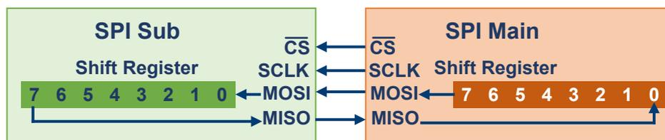
Figure 14-7: Simple configuration of SPI bus
