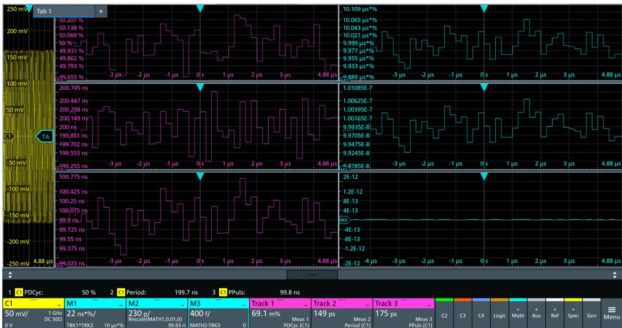
*Figure 10-6: Tracks used in math functions*
