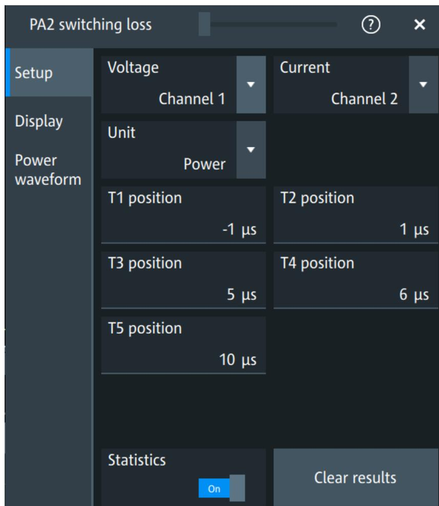
In the "Setup" tab, you configure the switching loss measurement: select the sources, the time points of the switching loss cycle, and if you want to measure either power or energy.
