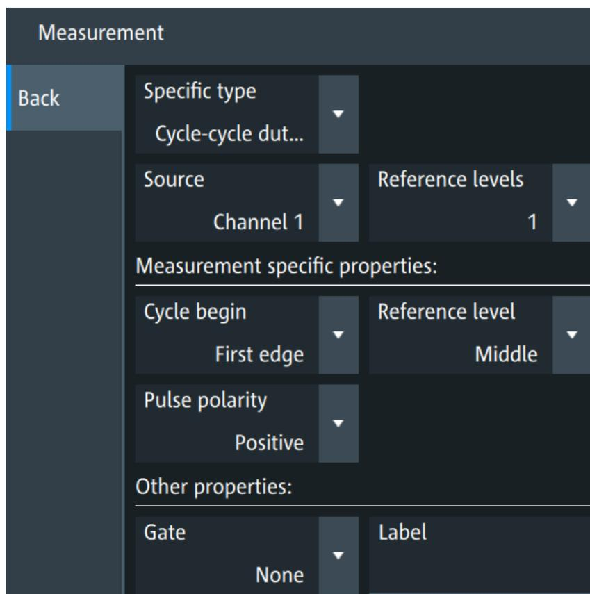
Figure 10-1: Setup for cycle-cycle duty cycle measurement
