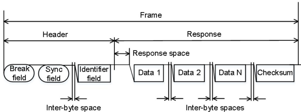
Figure 14-32: LIN frame with header and response
