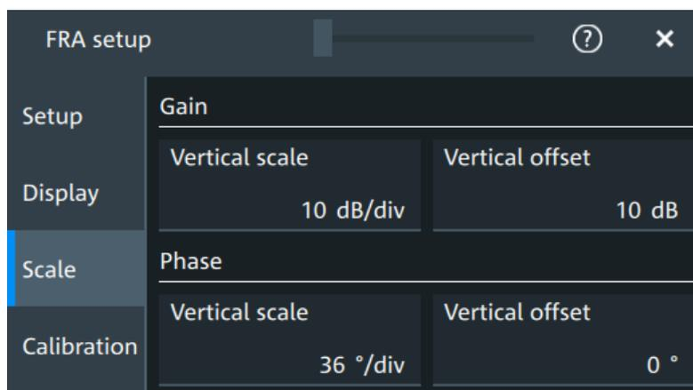
Figure 12-3: Scale dialog for Mode = Gain/Phase
