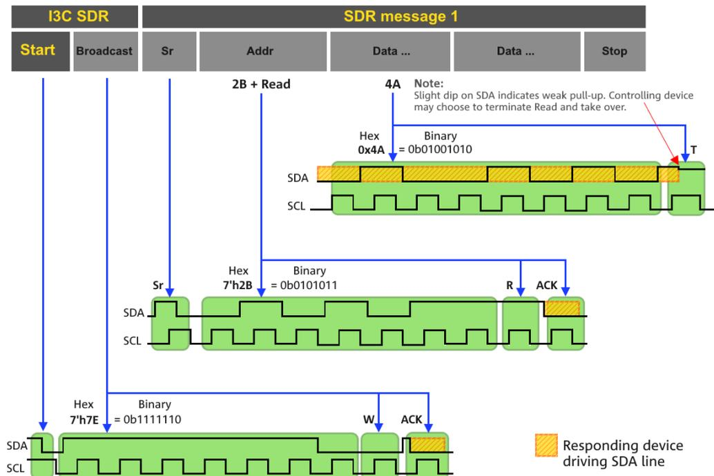
Figure 14-16: Example of using I3C coding SDR
