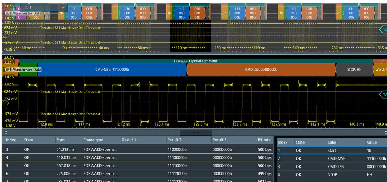
Figure 14-27: Decoded Manchester signal
