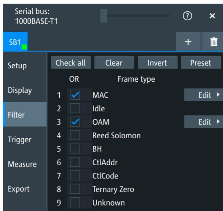
In the "Filter" tab, you can define the settings to display only the frames that match the selected filter conditions.
