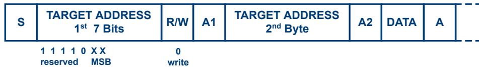
Figure 14-12: 10-bit address, write access
