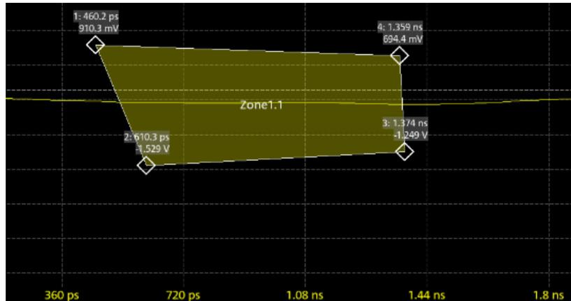
Figure 7-11: 1 area of a trigger zone
