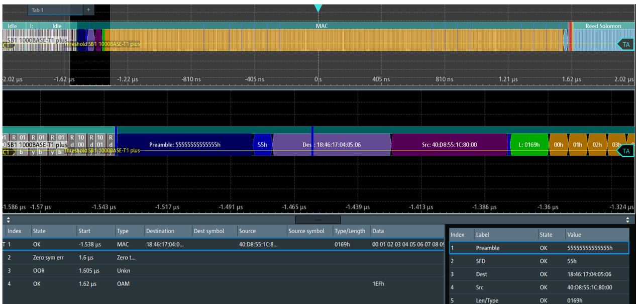
**Figure 14-53: Decoded 1000BASE-T1 signal**
