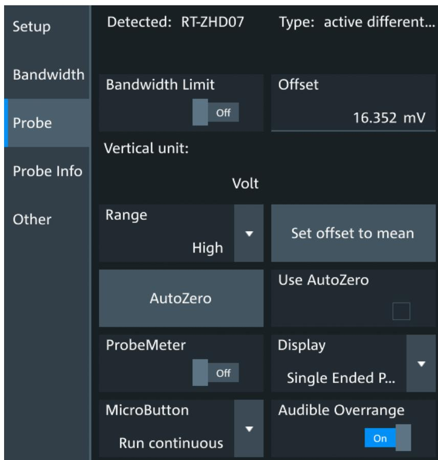
Figure 6-6: Setup for high-voltage differential probe R&S RT-ZHD07
