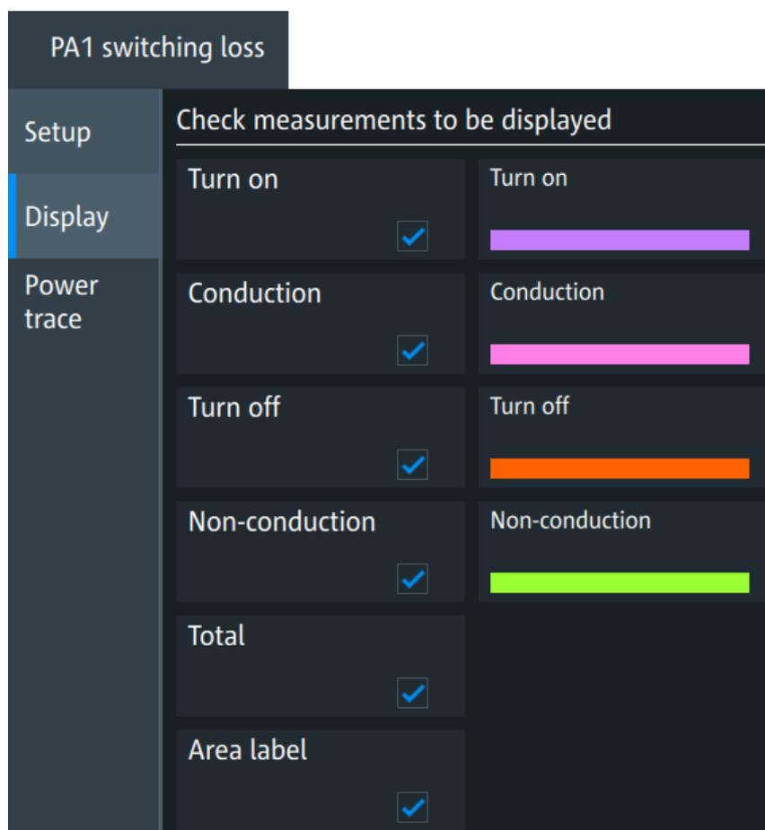
In the "Display" dialog, you select which measurements are performed. The results are displayed in the result table. You can change the colors of the cycle areas in the diagram.
