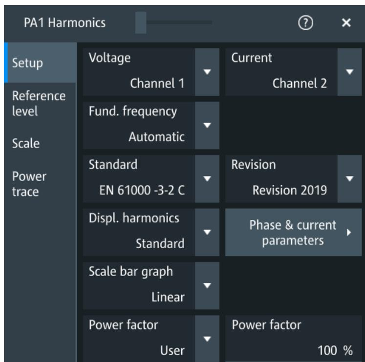
Figure 12-6: Power harmonic setup for EN 61000-3-2 C
