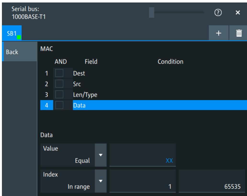
"Field" Enables the field type that you want to filter on for the selected frame. The available fields are "Dest", "Src", "Len/Type", "Data" and "OAM".
