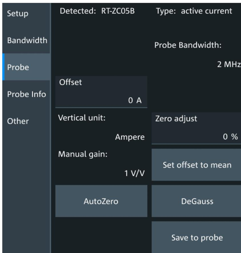
Figure 6-7: Setup for current probe R&S RT-ZC05B
