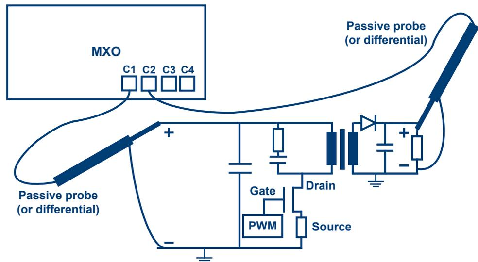
Figure 12-10: Connection with DC input
