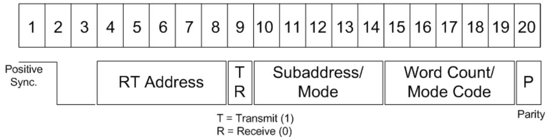
**Figure 14-43: Structure of a command word**
