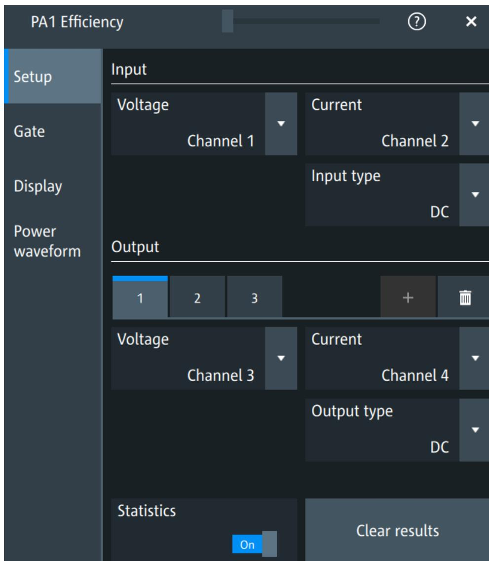
Figure 12-11: Efficiency measurement setup of an 8-channel instrument
