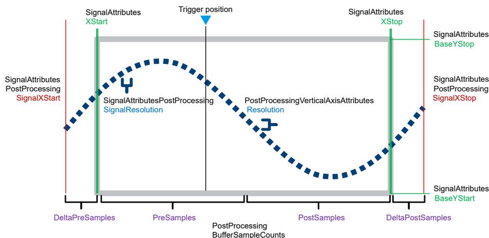
Figure 13-15: Main header properties at the waveform
