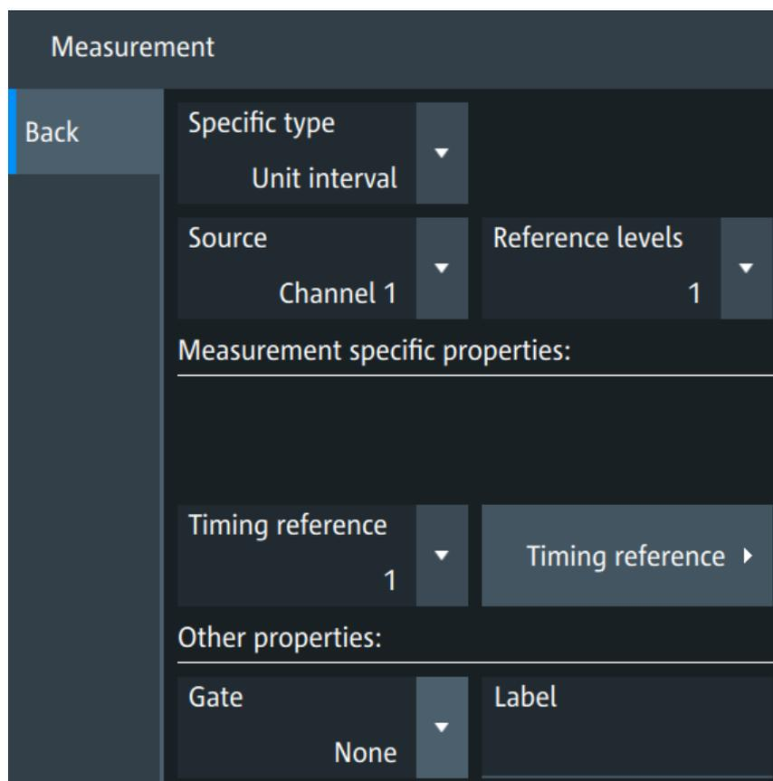
Figure 10-2: Setup for unit interval measurement
