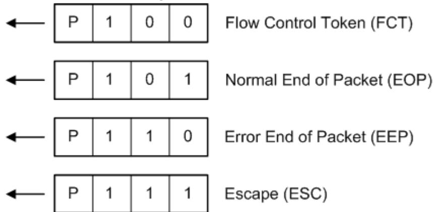
Figure 14-40: SpaceWire control characters
