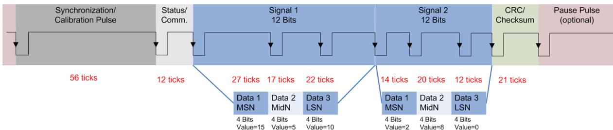
**Figure 14-34: Example of a SENT transmission sequence**
