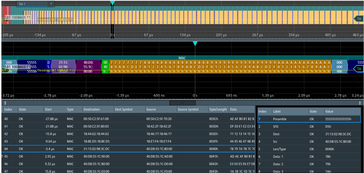
Figure 14-52: Decoded 100BASE-T1 signal
