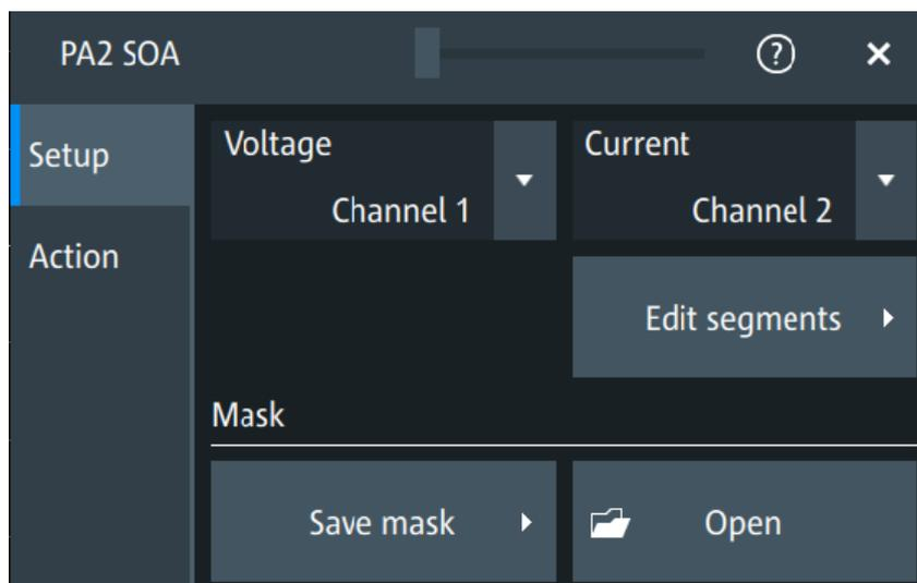
In the "Setup" tab, you configure the SOA measurement: select the sources, load and save the mask, and start creating a mask.
