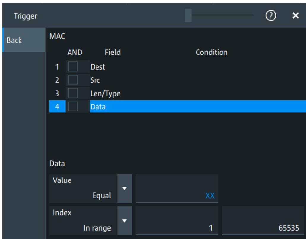
"Field" Enables the field type that you want to trigger on for the selected frame. The following fields are available: "Dest", "Src", "Len/Type", "Data".
