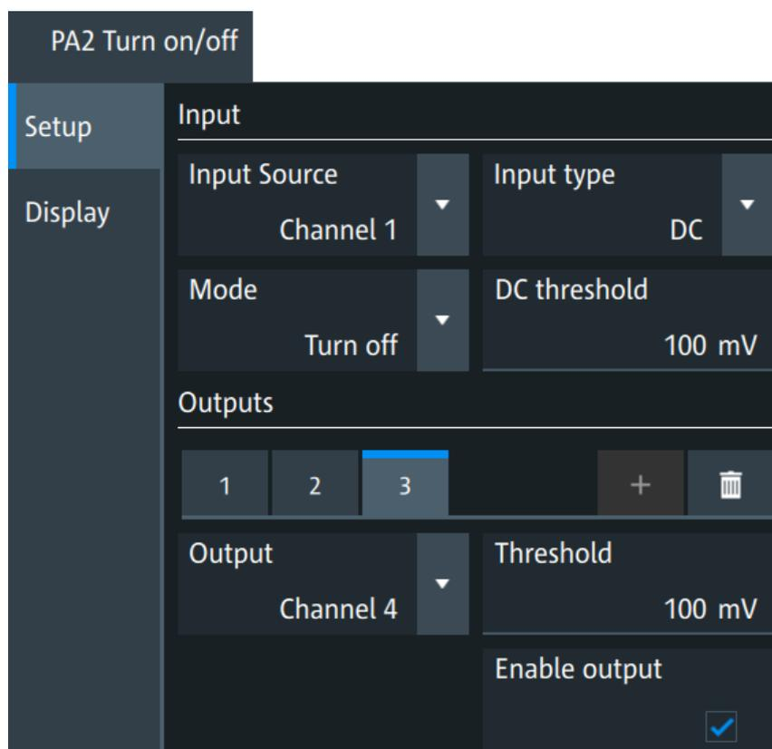
In the "Setup" tab, you configure the turn-on/off time measurement: select the sources, the thresholds, and the measurement.
