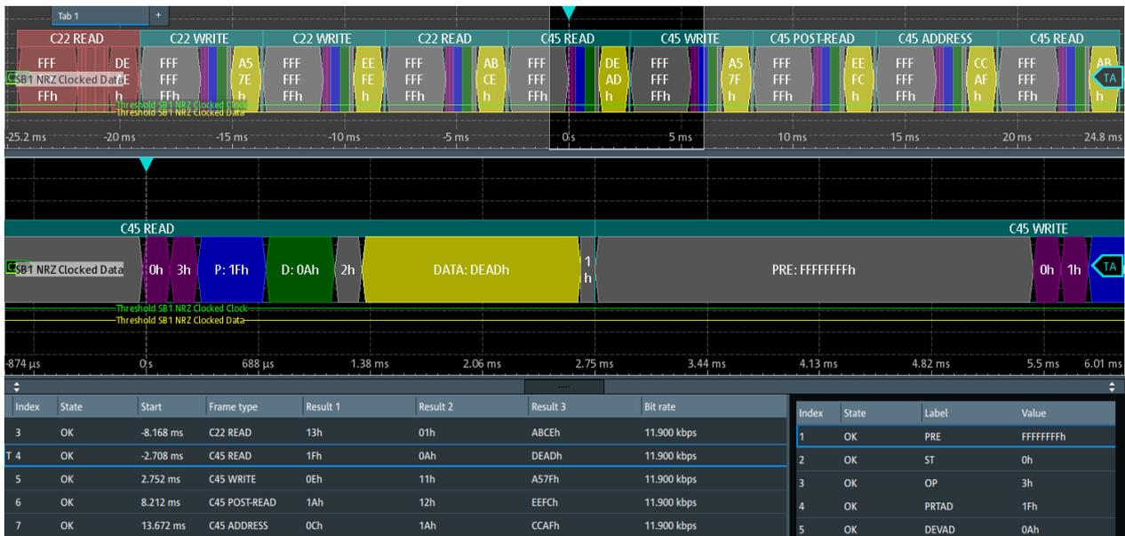
Figure 14-23: Decoded NRZ clocked signal
