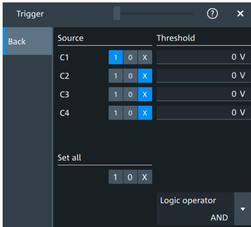
Figure 7-4: Detailed settings for pattern trigger
