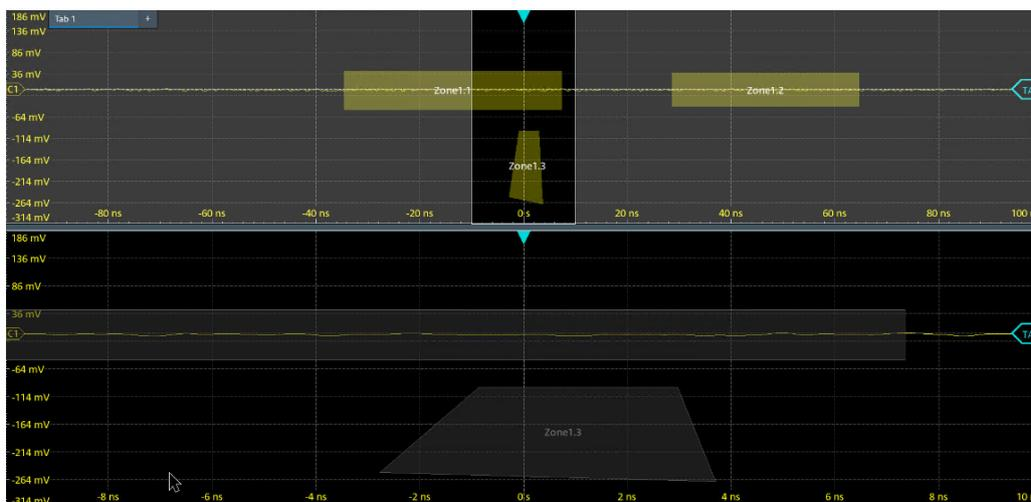
Figure 7-10: Trigger zone and a zoom diagram
