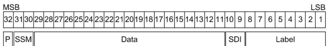
Figure 14-37: Structure of an ARINC 429 word
