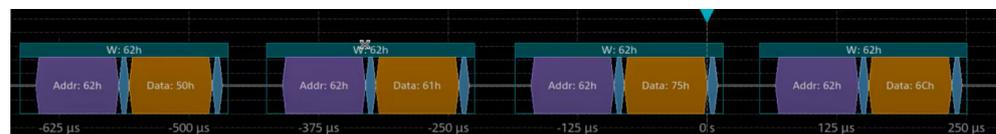
Figure 14-15: Trigger on Type=Data, Data=0x75 and Position=1
