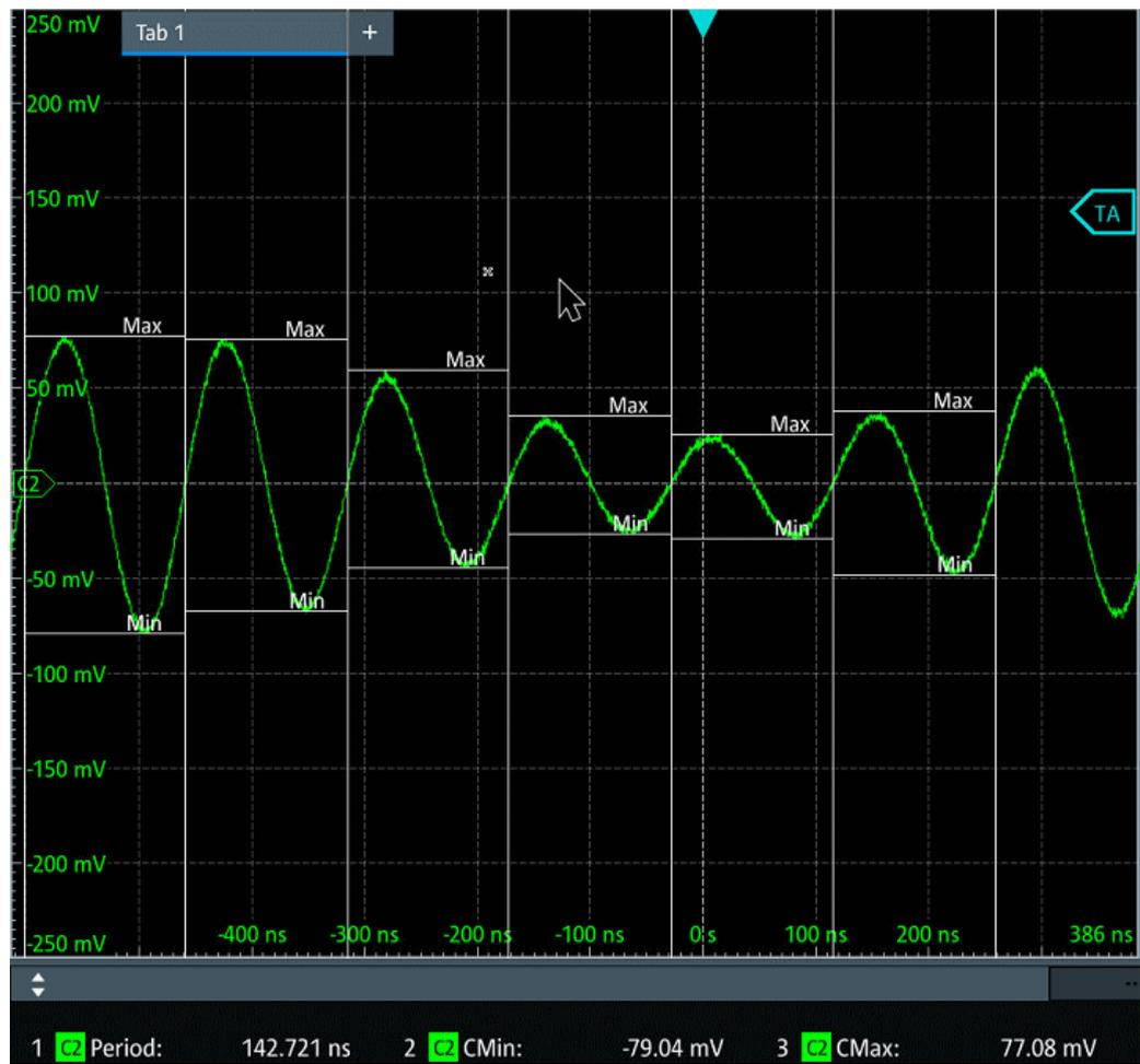
Figure 10-3: Example of annotations for cycle measurements
