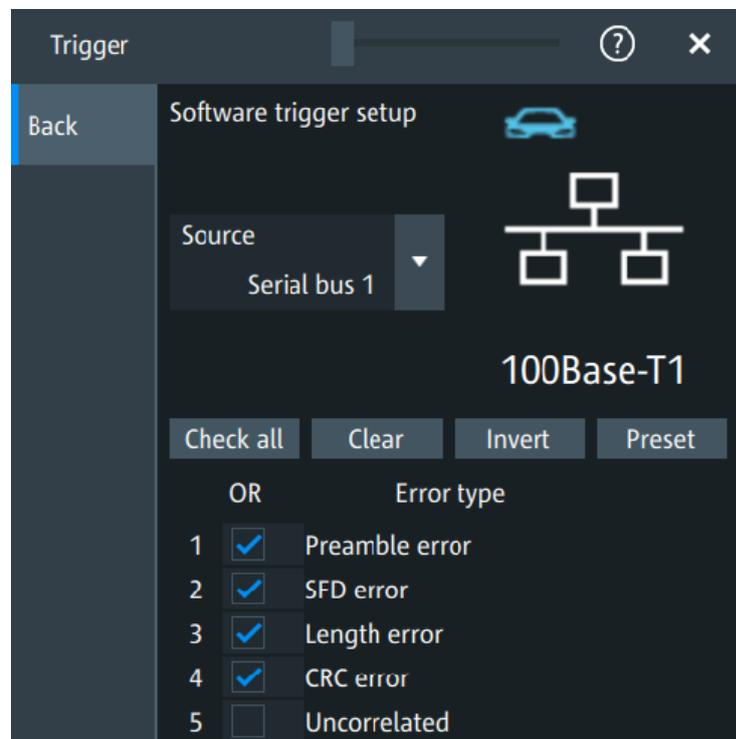
The following error types are available: "Preamble error", "SFD error", "Length error", "CRC error", "Uncorrelated".
