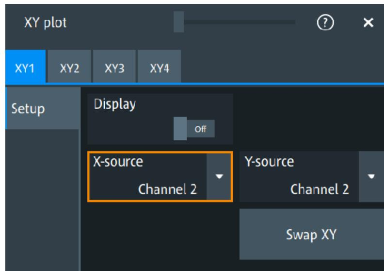
You can display up to four different XY-plots that use the voltage level of a waveform as the x-axis, rather than a time base.
