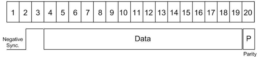
**Figure 14-44: Structure of a data word**
