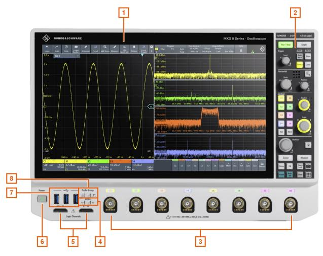
Figure 5-1: Front view of MXO 5 with 8 input channels
