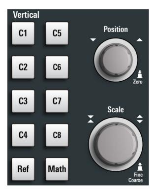
Figure 5-5: Vertical controls of MXO 5 with 8 input channels
