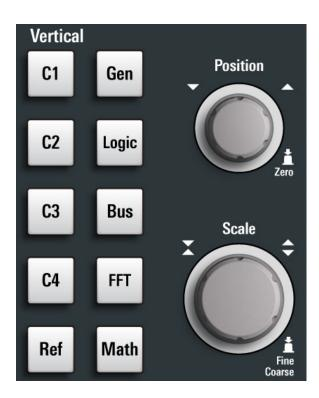
Figure 5-4: Vertical controls of MXO 5 with 4 input channels
