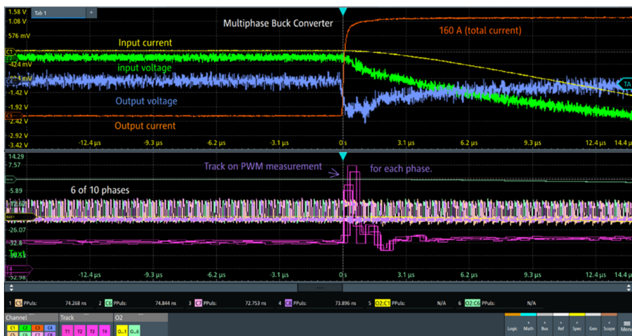
Figure 17-1: Example: analysis of multi-phase buck converter on MXO 5 with ScopeSync
