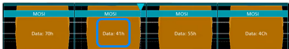
Figure 14-9: Trigger on Type= MOSI, Data pattern = 41
