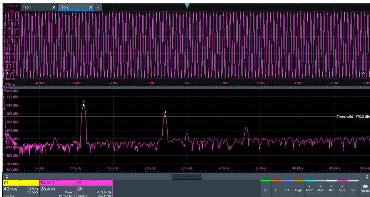
Figure 10-7: Track and spectrum on this track. C1 is not in the diagram.
