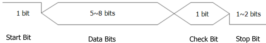
Figure 5-13 Schematic Diagram of RS232 Protocol
