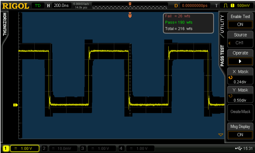
Figure 3-27 Pass/Fail Test of Frequent Abnormal Signal
