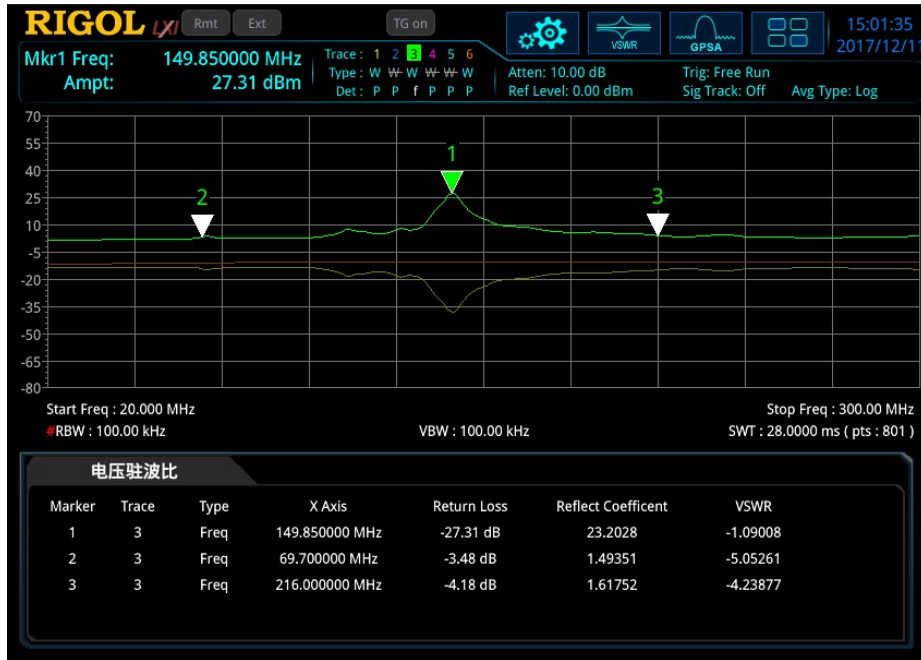
Figure 2-13 VSWR Measurement Interface
