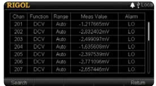
Multiple/All Channel Monitor
