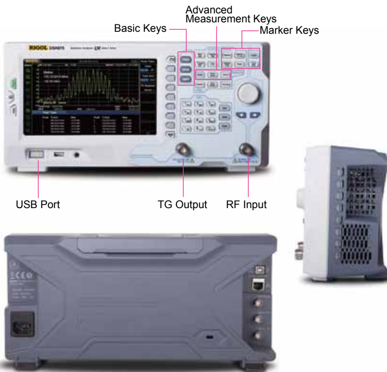
Product Dimensions: Width X Height X Depth = 361.6 mm x 178.8 mm x 128 mm
