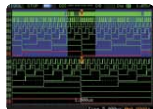
Duration Trigger A combination of Pattern Trigger and Pulse Width Trigger capabilities make isolation of events easy
