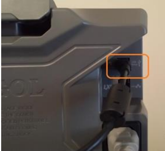
Figure 2: USB connection to DS1000Z series scope
