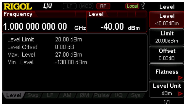
Figure 9 Parameter Setting Interface of RF Signal Output
