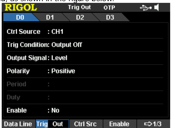
Figure 2-7 Trigger Output Setting Interface
