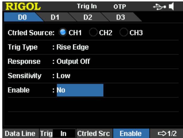
Figure 2-6 Trigger Setting Interface
