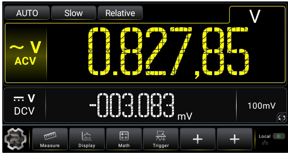
Figure 5.37 Main and Secondary Display Areas
