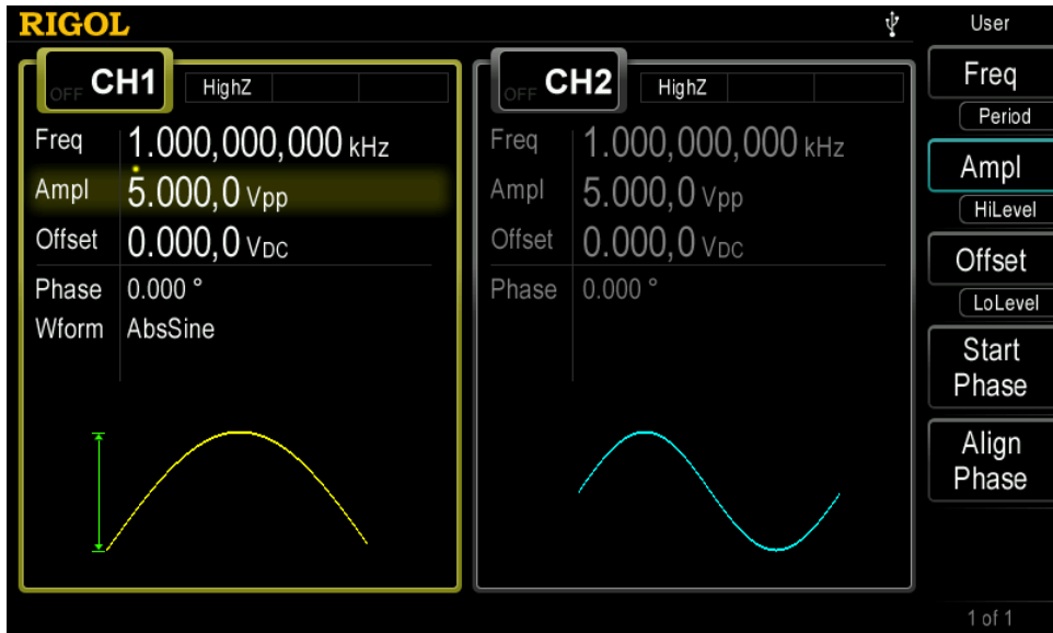
Figure 10-6 Press User Key to Quickly Edit Waveform Parameters
