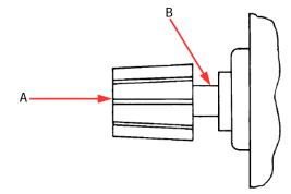
Method 1: Connect the test lead to A of the output terminal.
