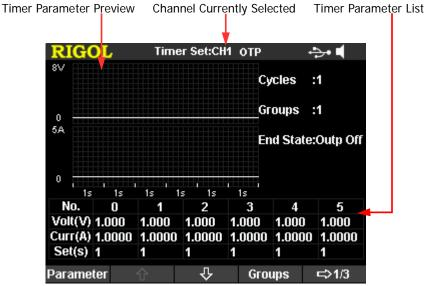
Figure 2-2 Timer Parameter Setting Interface
