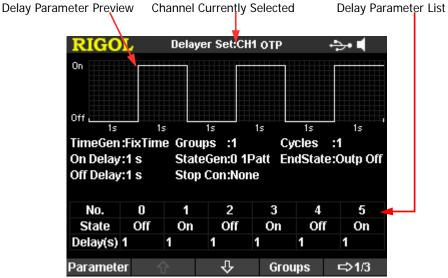
Figure 2-4 Delay Parameter Setting Interface
