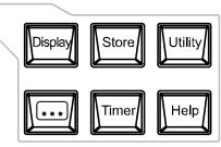
Press this key to enter the display parameter setting interface. Users can set the brightness, contrast, RGB luminance and display mode. Besides, you can also define the start-up interface.
