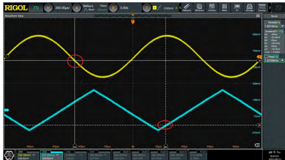
Figure 10.14 Track Measurement (after Horizontal Expansion)
