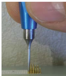
Termination being set FLUSH with an ITR-FL tool.
